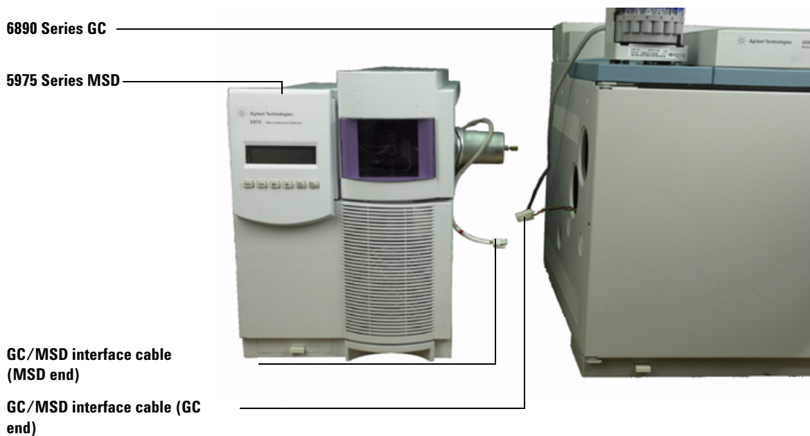
Figure 8 Connecting the MSD and the GC
